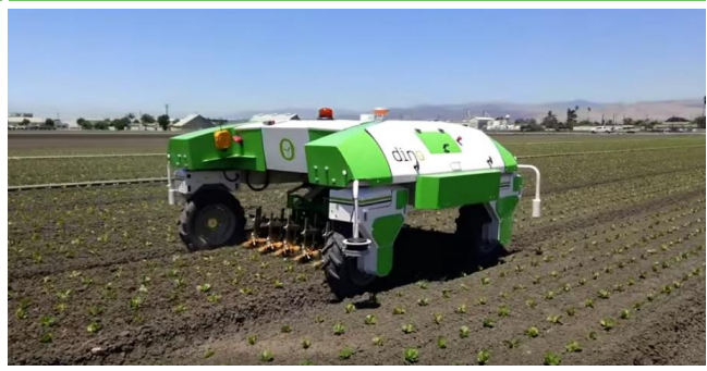
Exhibit 5: Video showing weeding robot in action
