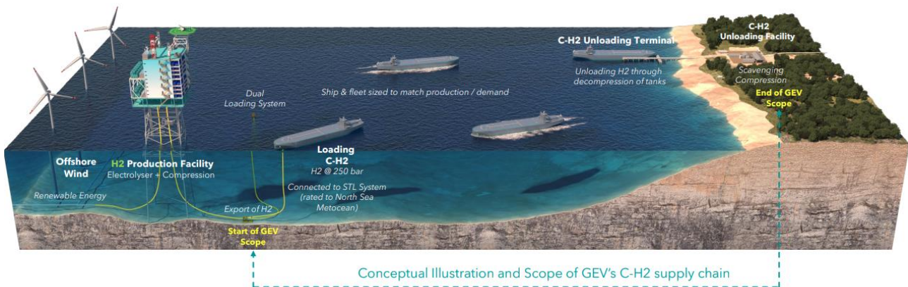
Exhibit 1: GEV's offshore green hydrogen C-H2 Ship solution
